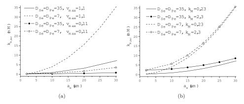
Fig. 2. Dependence of the apparent Michaelis constant of one-layer biosensor on the thickness of the enzyme membrane. (a)  $k_M = 0.23 \text{ mM}$ ; (b)  $v_{\text{max}} = 1.1 \text{ mM/s}$ .
