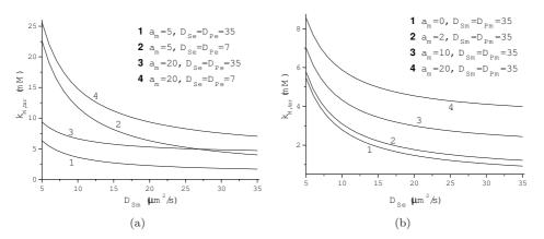
Fig. 3. Dependence of the apparent Michaelis constant of two-layer biosensor on the diffusivity in diffusion layer  $D_{S_m} = D_{P_m}$  (a) and in enzyme membrane  $D_{S_e} = D_{P_e}$  (b) at  $a_e = 10 \ \mu\text{m}$ ,  $k_M = 0.23 \ \text{mM}$  and  $v_{\text{max}} = 1.1 \ \text{mM/s}$ .
