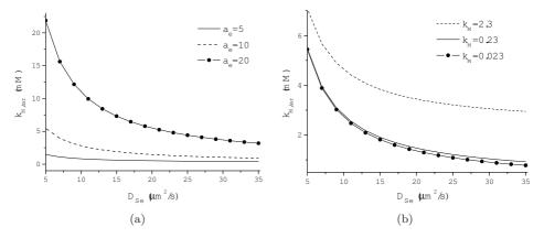
Fig. 1. Dependence of the apparent Michaelis constant of one-layer biosensor on the substrate diffusivity. (a)  $k_M = 0.23$  mM,  $v_{\text{max}} = 1.1$  mM/s; (b)  $a_e = 10 \text{ }\mu\text{m}$ ,  $v_{\text{max}} = 1.1$  mM/s.
