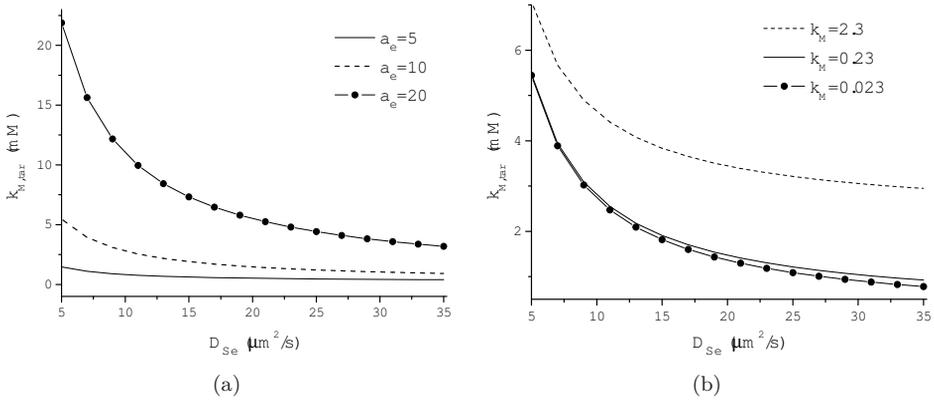
**Fig. 1.** Dependence of the apparent Michaelis constant of one-layer biosensor on the substrate diffusivity. (a)  $k_M = 0.23$  mM,  $v_{max} = 1.1$  mM/s; (b)  $a_e = 10$   $\mu\text{m}$ ,  $v_{max} = 1.1$  mM/s.
