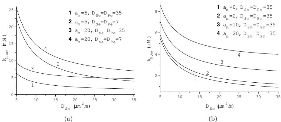
**Fig. 3.** Dependence of the apparent Michaelis constant of two-layer biosensor on the diffusivity in diffusion layer  $D_{S_m} = D_{P_m}$  (a) and in enzyme membrane  $D_{S_e} = D_{P_e}$  (b) at  $a_e = 10$   $\mu\text{m}$ ,  $k_M = 0.23$  mM and  $v_{\text{max}} = 1.1$  mM/s.
