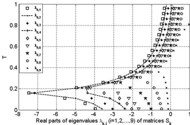
Fig. 3. Dependence of the real parts of the eigenvalues  $\lambda_{k,i}$  of matrices  $S_k$  on magnitude of delay  $T$  (matrices  $A$  and  $B$  are of ninth order).
