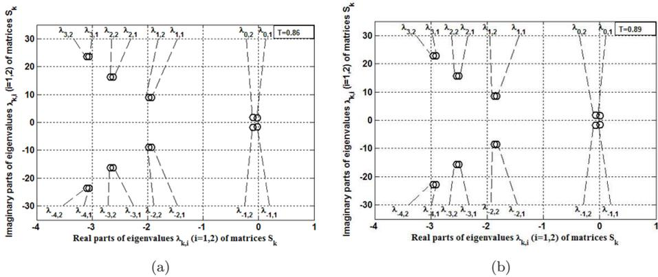
**Fig. 1.** Representation of the eigenvalues  $\lambda_{k,i}$  of matrices  $S_k$  ( $k = 0, \pm 1, \pm 2, \dots, i = 1, 2$ ) on the complex plane: (a) real parts of all eigenvalues are negative – corresponding dynamical system is asymptotically stable; (b) real parts of eigenvalues  $\lambda_{0,1}$  and  $\lambda_{-1,1}$  are positive – corresponding dynamical system is not stable.
