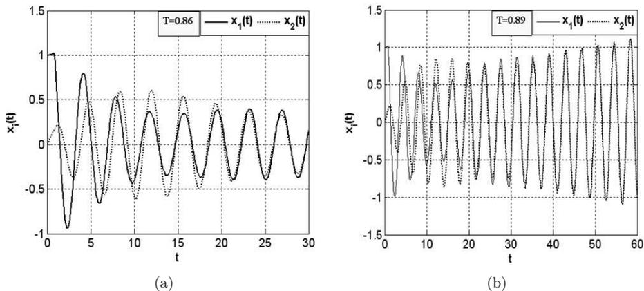
Fig. 2. Step responses of the system when the solutions of the corresponding matrix differential equation with delayed argument are: (a) asymptotically stable; (b) not stable.
