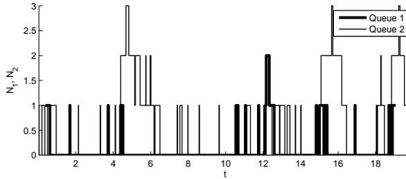
Fig. 2. The run of the  $M/G/2/\infty$  queuing system.
