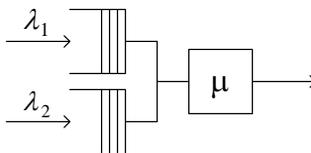
**Fig. 1.** The  $M/G/2/\infty$  queuing system with a priority.
