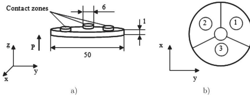
Fig. 1. Construction of mobile piezorobot.
