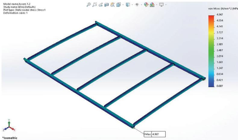
Fig. 5. Stress of the module in still water
