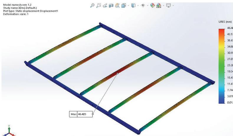
Fig. 6. Displacement of the module in still water
