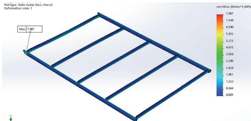
Fig. 7. Stress of the module in flowing water
