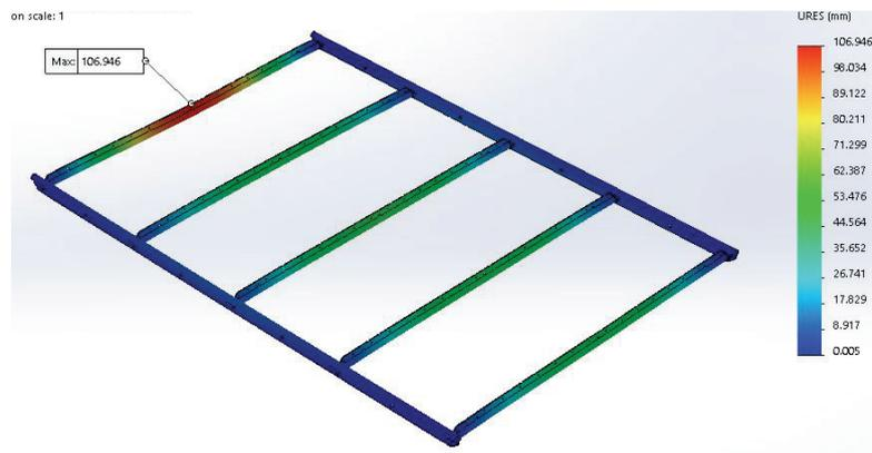
Fig. 8. Displacements of the module in flowing water
