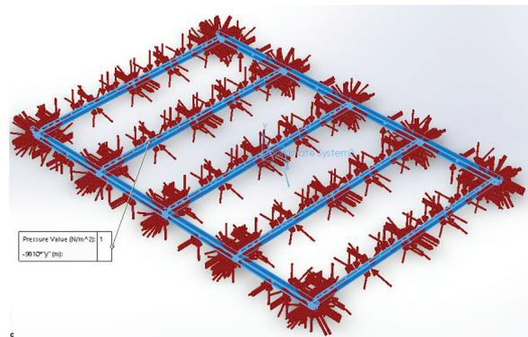
Fig. 4. Loads applied to the Structure
