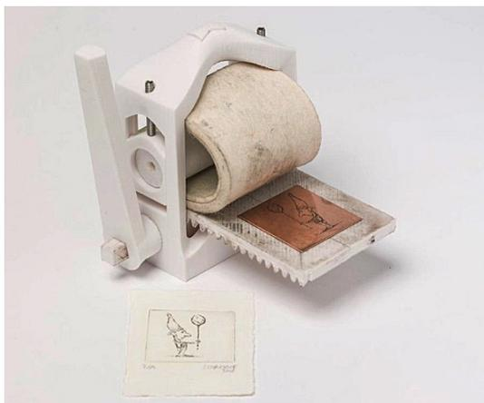
FIGURE 7: 3D printed and assembled Open Press with a completed engraved print.<sup>39</sup>
