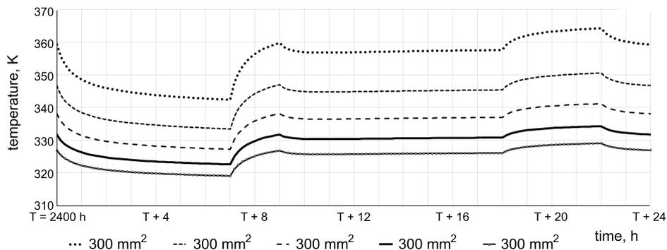
Figure 5. The daily dynamics of temperature in the conductor region of the central cable for different cable cross sections  $S$ .
