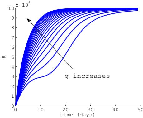
Fig. 8. Convergence rate variation due to changes in the gain  $g$ .
