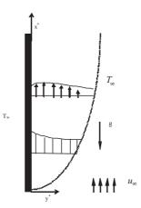
Fig. 1. The transient free convection model for a viscoelastic fluid near a vertical wall.
