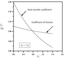
Fig. 6. Transient local coefficient of friction and local Nusselt numbers for different viscoelastic parameters.
