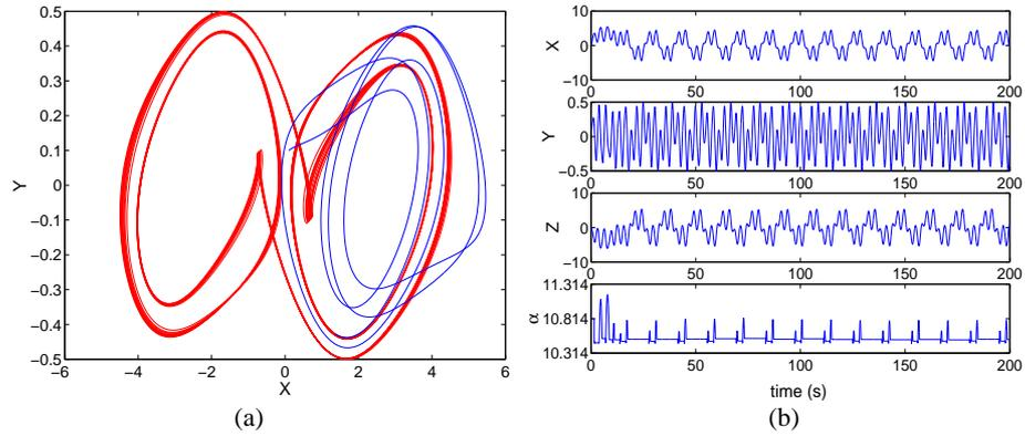
Fig. 3. Stabilizing the first UPO of the 8-scroll Chua's chaotic attractor: (a) phase space; (b) time response.
