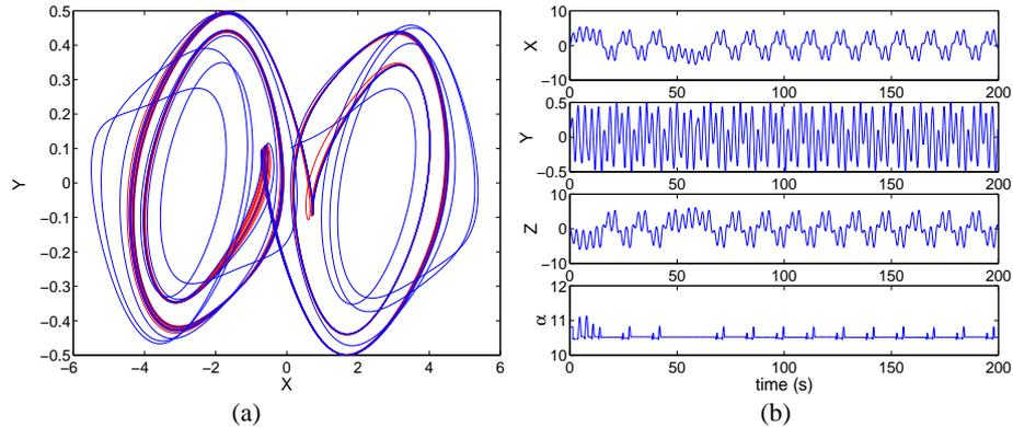
Fig. 7. The effect of noise on the controlled 8-scroll Chua's attractor.
