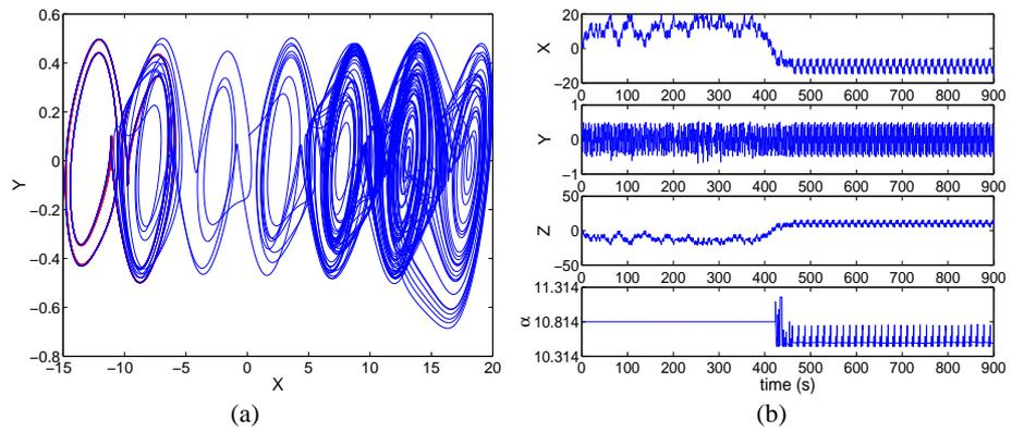
Fig. 5. Stabilizing the last UPO: (a) phase space; (b) time response.
