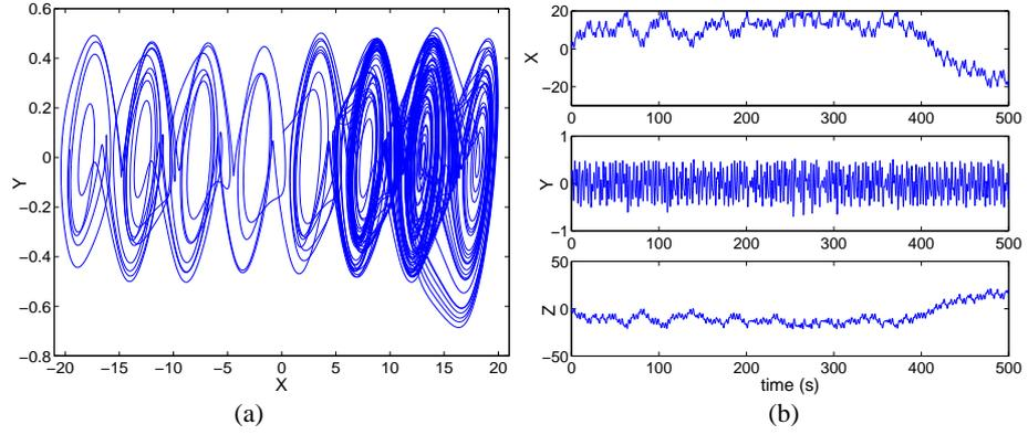
Fig. 1. The 8-scroll Chua's attractor: (a) phase space; (b) time response.
