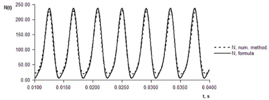
Fig. 9. The asymptotic stable solution of the differential equation (3), when  $h_N = 0.001 \text{ s}$ ,  $N_0 = 100 \text{ kW}$ ,  $r_N = 1800$ .
