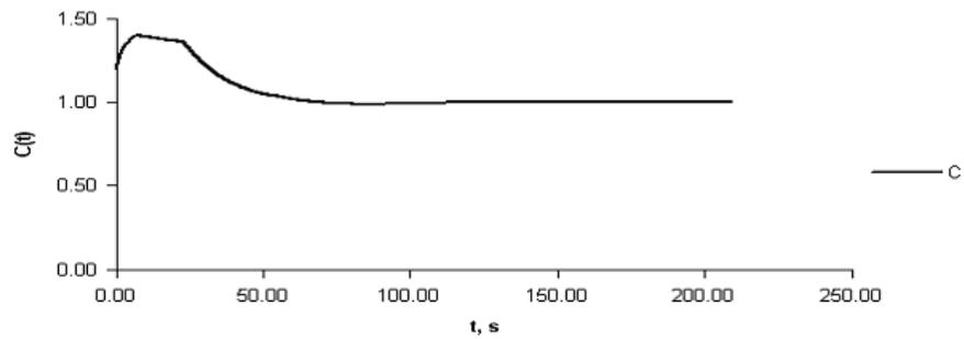
Fig. 6. The asymptotic stable solution of the differential equation (4), when  $N_0 = 100$  kW,  $C_0 = 1$  kW,  $r_C = 0.05$ .
