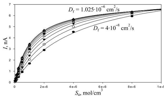
Fig. 3. Theoretical (points) and approximated by hyperbolas responses of the plate-gap electrode for different values of  $D_f$  (the numerical values and corresponding symbols as in Fig. 2);  $d_x \approx 0.002$  cm.
