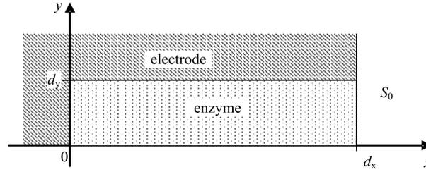
Fig. 1. The profile of the biosensor electrode.
