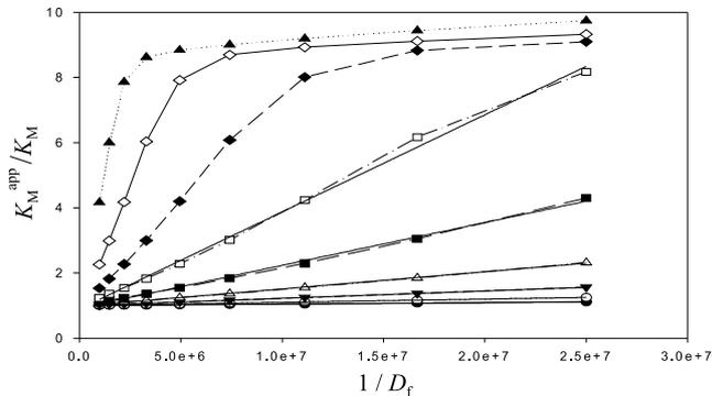
Fig. 6. Dependences of dimensionless parameter  $K_M^{app}/K_M$  on parameter  $1/D_f$  for different values of  $d_x$ : 0.0004 (●), 0.0006 (○), 0.0009 (▼), 0.00135 (▽), 0.002 (■), 0.003 (□), 0.0045 (◆), 0.0068 (◇), 0.01 (▲) cm.
