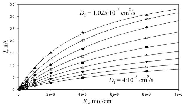
Fig. 4. Theoretical (points) and approximated by hyperbolas responses of the plate-gap electrode for different values of  $D_f$  (the numerical values and corresponding symbols as in Fig. 2);  $d_x \approx 0.01$  cm.
