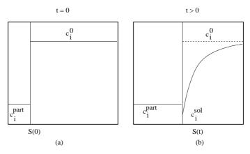
Fig. 4. The hypothetical case  $c_i^{\rm sol} < c_i^{\rm part} < c_i^0$  which gives growth of the  $\alpha$ -phase and violation of the mass-balance. Left (a) shows the initial situation and right (b) shows a hypothetical (but impossible) situation at some time t > 0.
