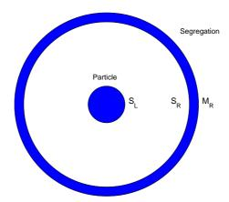
Fig. 11. The geometry of a grain with a Si-particle in the center and a Mg<sub>2</sub>Si-segregation at the grain boundary.
