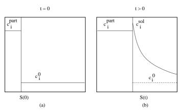
Fig. 3. The hypothetical case  $c_i^0 < c_i^{\rm part} < c_i^{\rm sol}$  which gives growth of the  $\alpha$ -phase and violation of the mass-balance. Left (a) shows the initial situation and right (b) shows a hypothetical (but impossible) situation at some time t>0.
