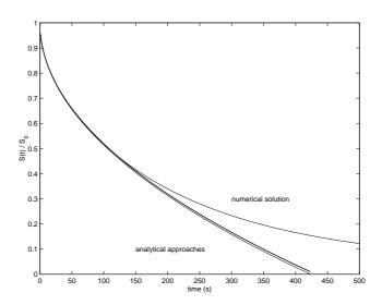
Fig. 8. The interface position as a function of time during the dissolution of a planar phase. The top curve represents the solution obtained by the Finite Difference method with an finite volume of the cell. The other curves represent the analytical approaches for the infinite volume of the cell, where the lowest curve represents the quasi-binary approach and the other curve represents the full multi-component "analytical" solution where a zero-point method is used.
