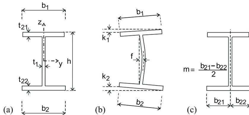
Fig. 3. Initial geometrical imperfections of the beam section.
