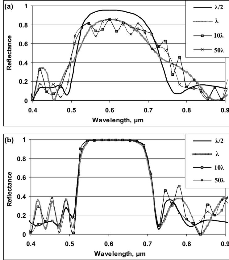
Fig. 1. Reflectivity spectra of DBR mirror, when thickness of the AL is  $\lambda/2$ ,  $\lambda$ ,  $5\lambda$ ,  $10\lambda$ ,  $50\lambda$  and its refraction index is  $n_0 = 1.5$ . Refraction indexes of Bragg mirrors  $\lambda_c/4$  layers are  $n_1 = 2.25$  and  $n_2 = 1.5$  and the number of layers: (a)  $i_p = 0$ ,  $i_g = 8$ ; (b)  $i_p = 0$ ,  $i_g = 15$ ,  $\lambda = \lambda_c = 600$  nm.
