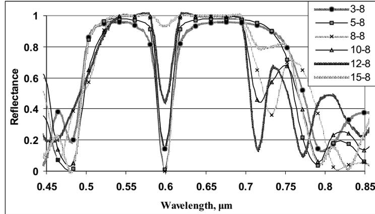
Fig. 2. Fabry-Perot microcavity reflectivity spectra, when the thickness of AL is  $\lambda$  and its refractive index  $n_0 = 1.27$ . Refractive indexes of layers of DBR mirrors are  $n_1 = 2.25$  and  $n_2 = 1.5$ . The number of layers –  $i_p = 3, 5, 8, 10, 12, 15$ ,  $i_g = 8$ ,  $\lambda_c = 600$  nm.
