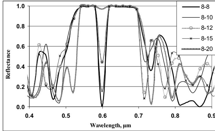
Fig. 3. Fabry-Perot microcavity reflectivity spectra, when the AL spacer thickness is  $\lambda$  and its refractive index  $n_0 = 1.27$ . Refractive indexes of layers of DBR mirrors are  $n_1 = 2.25$  and  $n_2 = 1.5$ . The number of layers –  $i_p = 8$ ,  $i_g = 8, 10, 12, 15, 20$ ,  $\lambda_c = 600$  nm.
