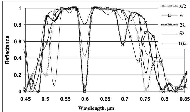
Fig. 4. Fabry-Perot microcavity reflectivity spectra, when  $\lambda_c = 600$  nm, the thickness of AL spacer is  $d = \lambda/2, \lambda, 2\lambda, 5\lambda, 10\lambda$ , and its refraction index  $n_0 = 1.27$ . The layer number in stacks of Bragg mirrors is  $i_p = i_g = 8$ , and their refraction indexes  $n_1 = 2.25$  and  $n_2 = 1.5$ .
