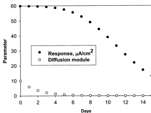
Fig. 3. The change of response and diffusion module of trienzyme biosensor during enzyme inactivation. Life-time of  $E_1$  was 2 days, other parameters as in Fig. 1.
