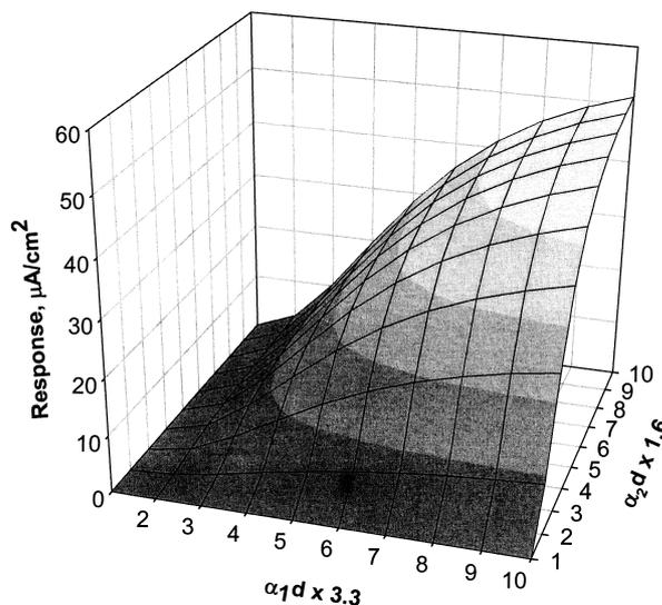
Fig. 2. The dependence of biosensor response on diffusion modules  $\alpha_1 d$  and  $\alpha_2 d$ . For calculations  $s_0 = 1 \mu mol/cm^3$  and  $\alpha_3 d = 10.3$  was used.
