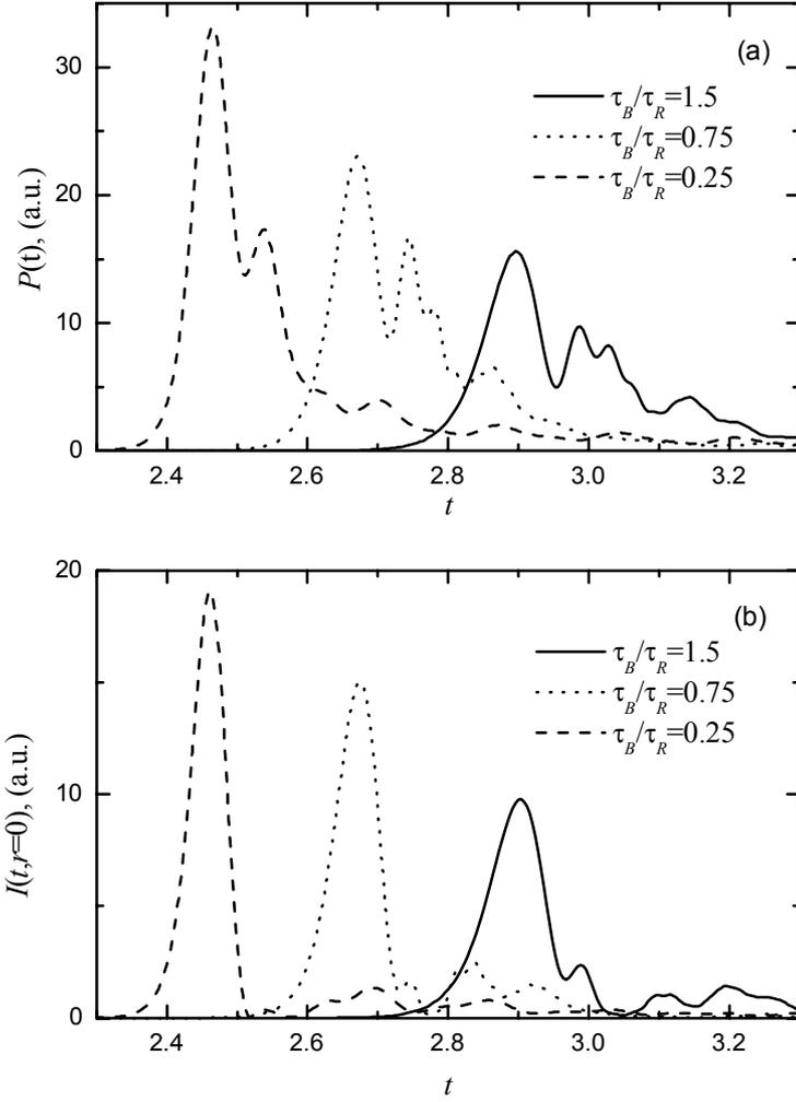
**Fig.6.** Temporal dependences a) of the instantaneous power  $P(t)$  and b) of the intensity on the beam axis  $I(t, r = 0)$  of the Stokes pulse at the cell output upon the hypersound wave period  $T_B$  at the input laser pulse energy  $E_{L0} = 12$  mJ, the duration  $T_{L0} = 1$  ns and constant lifetime  $T_R = 0.4$  ns.
