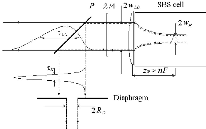
Fig.1 The optical scheme of an SBS compressor
