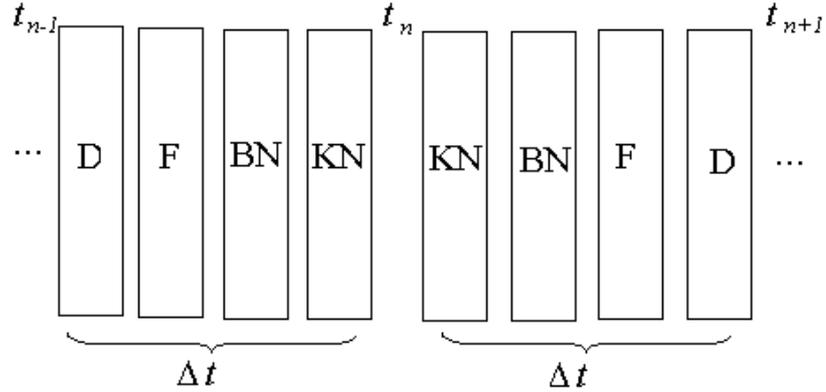
**Fig.2** The scheme of the numerical method,  $t_n = n\Delta t$ ,  $n = 0 \div N_T$ ,  $\Delta t N_T = t_m$
