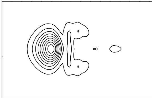
**Fig.3. Spatio-temporal structure of compressed Stokes pulses at the exit of SBS-cell for the input laser pulse with energy  $E_{L0} = 12$  mJ, duration  $T_{L0} = 2$  ns, hypersound wave period  $T_B = 0.75$  ns and its lifetime  $T_R = 0.4$  ns.**
