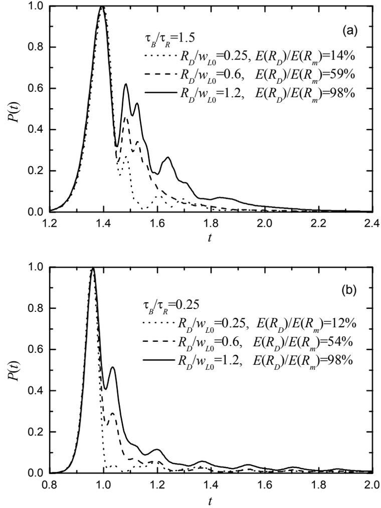
**Fig.7.** The envelopes of the instantaneous power  $P(t)$  of Stokes pulses propagated through diaphragms of different radii and the hypersound period  $T_B$  at the input laser pulse energy  $E_{L0} = 12$  mJ, the duration  $T_{L0} = 1$  ns, beam waist  $w_{L0} = 0.09$  cm and lifetime  $T_R = 0.4$  ns.
