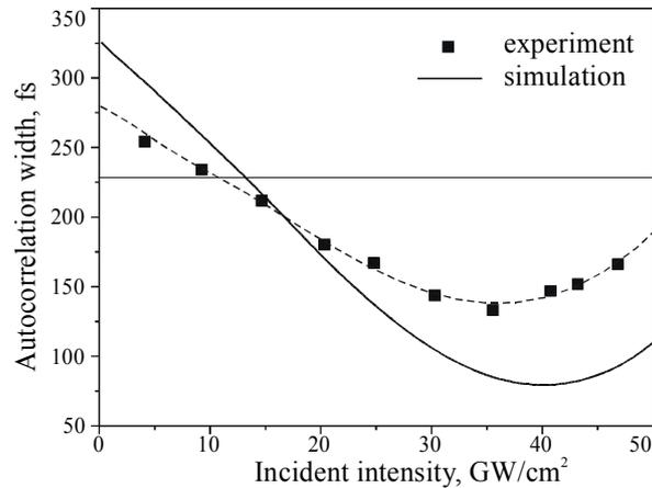
Fig. 6. Autocorrelation width dependence on the incident intensity.
