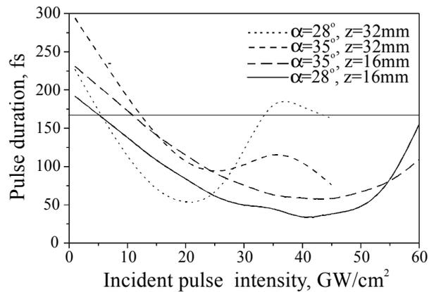
Fig. 2. Pulse duration dependence on the incident intensity for different pulse-front tilt angles and media length  $z$ .
