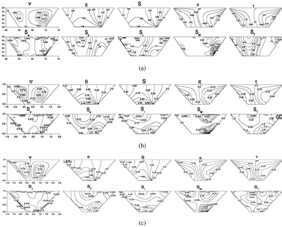
**Figure 4.** Stream lines ( $\psi$ ), isotherms ( $\theta$ ), isoconcentrations ( $S$ ), heat lines ( $\pi$ ), mass lines ( $\tau$ ), entropy generations due to fluid friction ( $S_\psi$ ), heat transfer ( $S_\theta$ ), mass transfer ( $S_\tau$ ) magnetic field ( $S_M$ ) and total entropy generation ( $S_T$ ) for  $Ra = 10^3$ ,  $Ha = 20$ ,  $N = 1$ ,  $Pr = 0.7$ ,  $Le = 2$  and  $\phi = 45^\circ$  for (a)  $A = 0.5$ , (b)  $A = 1.0$  and (c)  $A = 1.5$ .
