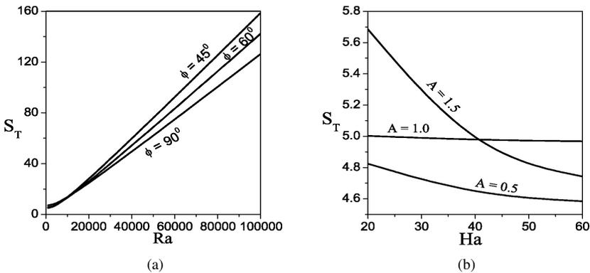
**Figure 8.** Variation of total entropy generation ( $S_T$ ) with  $Ra$  and  $Ha$  for different values of  $\phi$  and  $A$ , respectively, at  $Pr = 1000$ ,  $Le = 2$  and  $N = 1$ .
