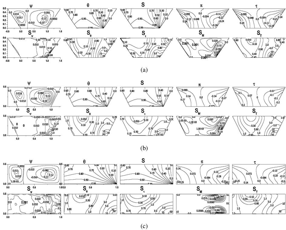
**Figure 5.** Stream lines ( $\psi$ ), isotherms ( $\theta$ ), isoconcentrations ( $S$ ), heat lines ( $\pi$ ), mass lines ( $\tau$ ), entropy generations due to fluid friction ( $S_\psi$ ), heat transfer ( $S_\theta$ ), mass transfer ( $S_\tau$ ) magnetic field ( $S_M$ ) and total entropy generation ( $S_T$ ) for  $Ra = 10^3$ ,  $Ha = 20$ ,  $N = 1$ ,  $Pr = 0.7$ ,  $Le = 1$  and  $A = 0.5$  for (a)  $\phi = 45^\circ$ , (b)  $\phi = 60^\circ$  and (c)  $\phi = 90^\circ$ .
