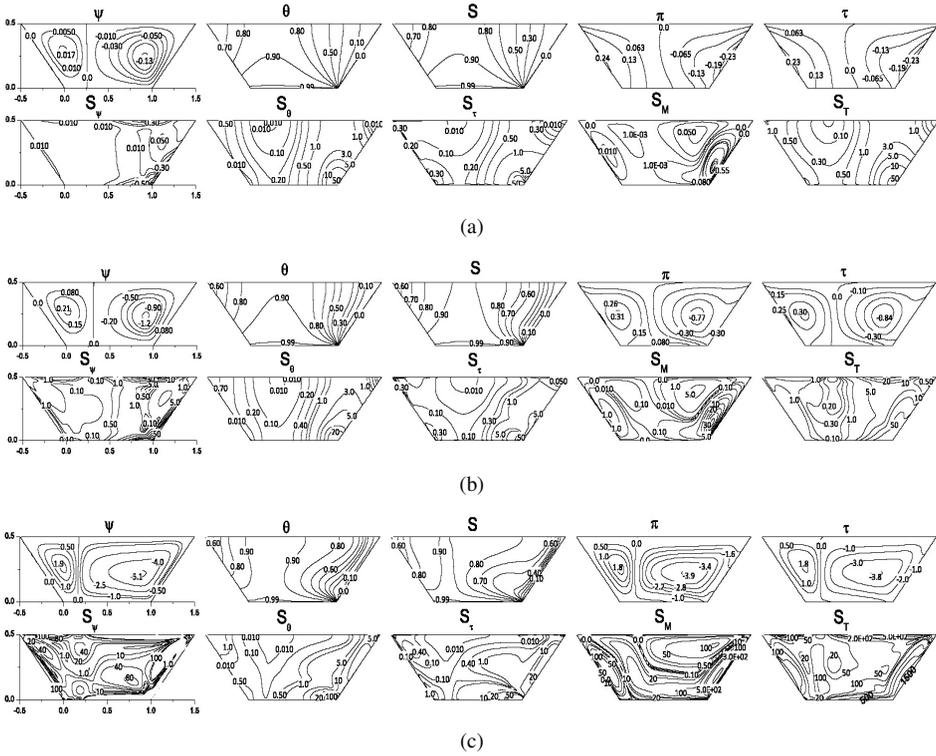
**Figure 6.** Stream lines ( $\psi$ ), isotherms ( $\theta$ ), isoconcentrations ( $S$ ), heat lines ( $\pi$ ), mass lines ( $\tau$ ), entropy generations due to fluid friction ( $S_\psi$ ), heat transfer ( $S_\theta$ ), mass transfer ( $S_\tau$ ) magnetic field ( $S_M$ ) and total entropy generation ( $S_T$ ) for  $\phi = 45^\circ$ ,  $Ha = 20$ ,  $N = 1$ ,  $Pr = 1000$ ,  $Le = 2$  and  $A = 0.5$  for (a)  $Ra = 10^3$ , (b)  $Ra = 10^4$  and (c)  $Ra = 10^5$ .
