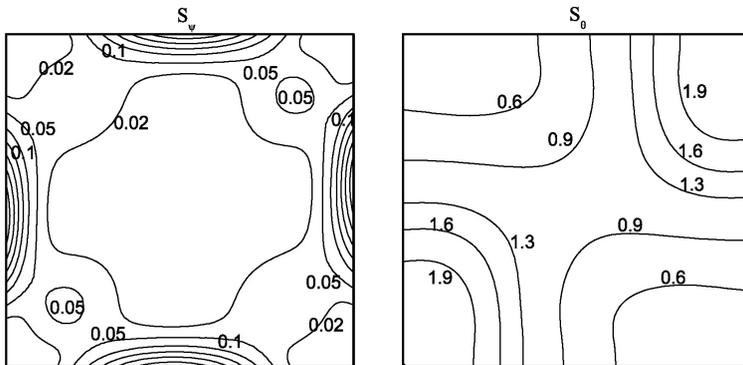
Figure 3. Entropy generation due to fluid friction ( $S_\psi$ ) and heat transfer ( $S_\theta$ ) contours within a square cavity with hot left side wall, cold right side wall, adiabatic top and bottom walls for  $Ra = 10^3$  and  $Pr = 0.7$ .
