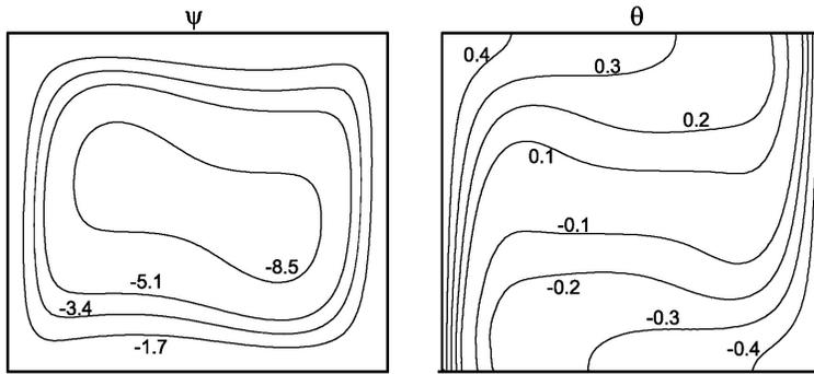
Figure 2. Stream function ( $\psi$ ) and isotherm ( $\theta$ ) contours within a square cavity with hot left side wall, cold right sidewall, adiabatic top and bottom walls for  $Ra = 10^5$  and  $Pr = 0.7$ .
