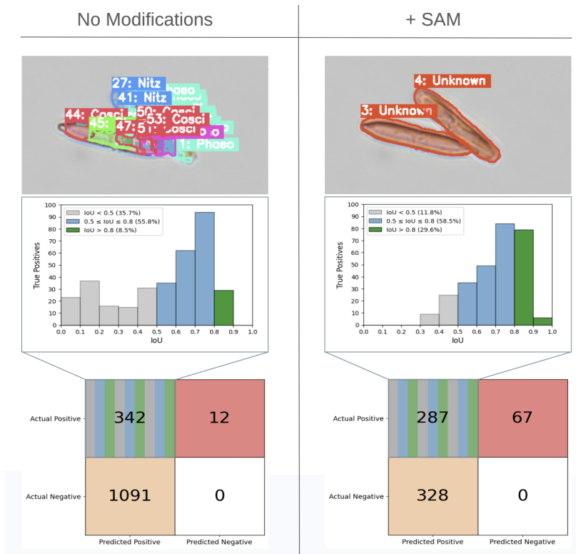
Figure 5. Top: Visual examples of Algvision (our pipeline) trying to identify and segment unknown strains before and after prompting the ViT-B SAM model; Middle: Count of true positives against their IoU distributions; Bottom: Confusion matrices of both approaches. Ground truth and prediction mask overlapping threshold (to be counted as true positive) > 0 IoU.
