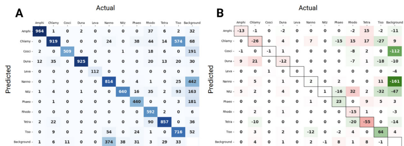
Figure 3. A: Confusion matrix of the prediction results on the test split. Blue shading indicates the number of occurrences. Ground truth and prediction mask overlapping threshold \geq 0.5 IoU; B: Confusion matrix of the change of test split predictions after custom post-processing. Green and red shading indicate improvement and error, respectively. Note that diagonal cells (borders highlighted) are true positives – increases in the number of cells counted are colored in green because that equals improvement.
